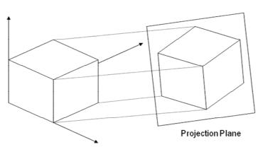
Figure 6.5: Axonometric projection
