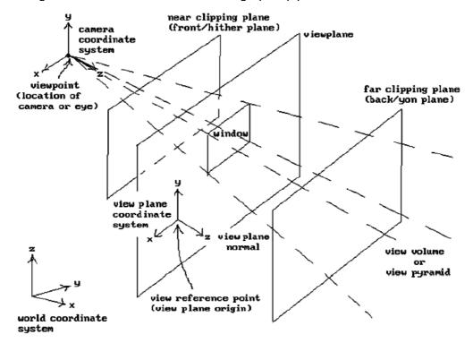
Figure 1.1: A 3D graphic pipeline
