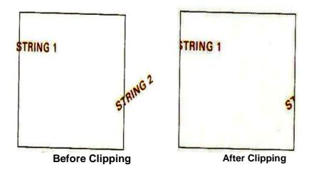
Text clipping is performed on the components of individual characters.
