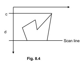
Here, all the pixels inside the polygon can be painted without leaving any of the neighboring pixels. If the point of intersection of an edge and the scanline is a vertex, we shorten one of the edges. So that it will be contributed to the intersection is 1. If the endpoint of the two edges are on one side of the scan line and the contribution will be 2 if the other points are on the opposite side of the scanline.
