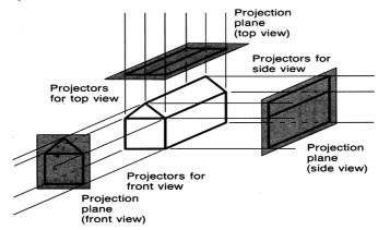
Figure 6.4: Views in orthographic projection
