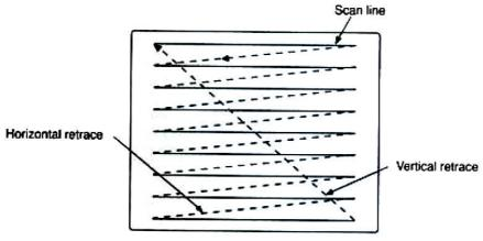
Figure 1.10 (showing horizontal and vertical retrace)
