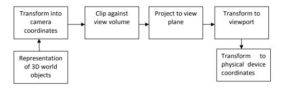
Figure : Sequence of transformation in viewing pipeline
