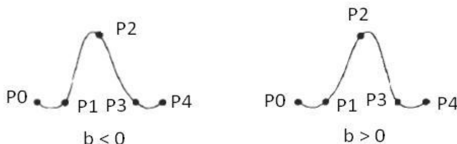
Fig. 4.19: -Effect of bias parameter on the shape of a Kochanek-Bartels spline section.
