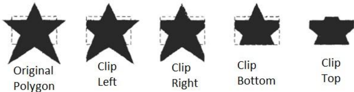
Fig. 3.11: - Clipping a polygon against successive window boundaries.
