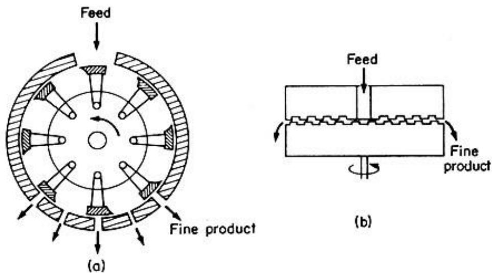
Figure 11.2 Grinders: (a) hammer mill, (b) plate mill
