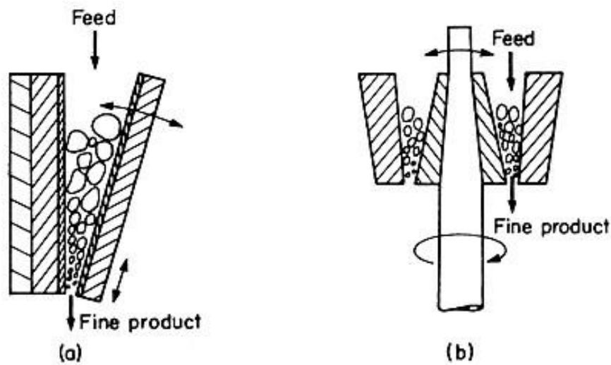
Figure 11.1 Crushers: (a) jaw (b) gyratory
