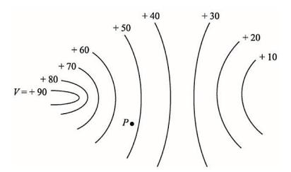
\*Equipotential surfaces shown as lines in the two dimensional sketch.
