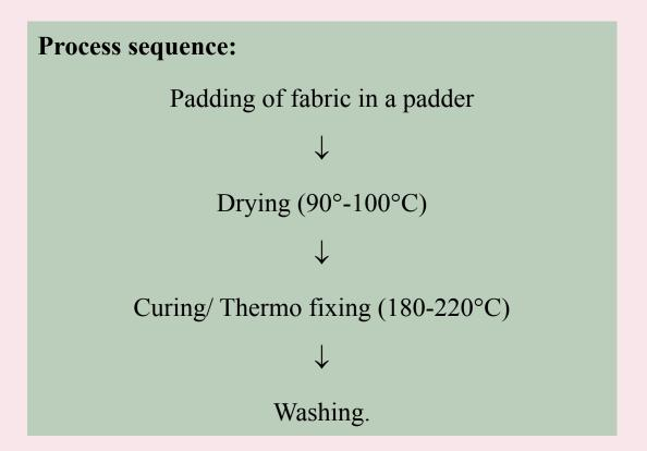
Mechanism of thermo sol Process: In thermosol process, dye is dissolved in fiber. But dye heat is used instead of aqueous medium. Dye is deposited on fiber surface. When fiber is exposed at dry heat temp (250°C), then dye is directly dissolved in fiber. Complete penetration is occurred at 60s.
