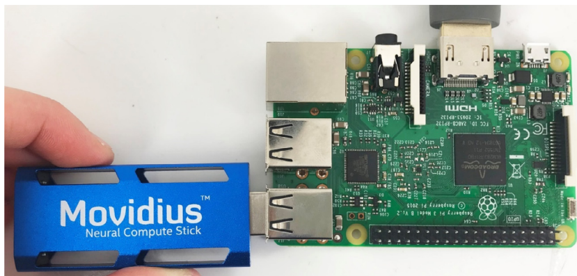
Fig. 9. The Movidius neural compute stick is a low-power and small form factor device that can implement deep neural network algorithms for signal processing and image recognition. Here, a Movidius compute stick costing $75 it is shown attached to a USB port of a Raspberry Pi Model 3-B that costs $35.
