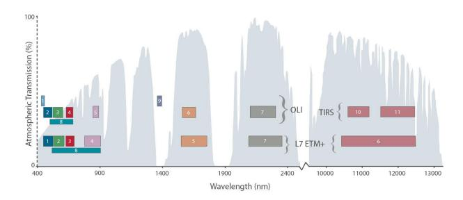
The OLI collects data for two new bands, a coastal/aerosol band (band 1) and a cirrus band (band 9), as well as the heritage Landsat multispectral bands. Additionally, the bandwidth has been refined for six of the heritage bands. The Thermal Instrument (TIRS) carries two additional thermal infrared bands. Note: atmospheric transmission values for this graphic were calculated using
