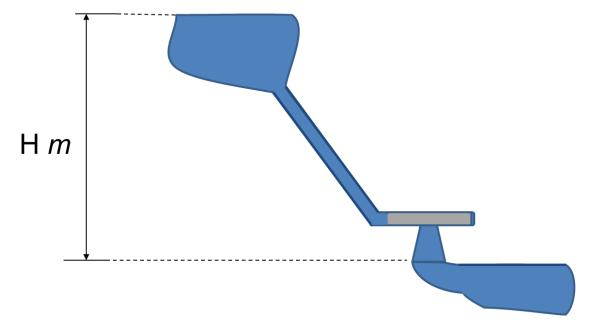
Hydroelectric power plants are usually located in dams that impound rivers, thereby raising the level of the water behind the dam and creating as high a head as is feasible. The potential power that can be derived from a volume of water is directly proportional to the working head, so that a high-head installation requires a
