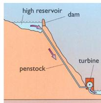
Low Head Plants: Low head plants have water head below 30 m. A low head power plant stores water by the construction of a dam or a barrage across a river and the power plant is installed near the base of the dam on the downstream side. Generally, one half of the barrage has regulating gates so that excess water is allowed to flow in the river from these gates to the river. Depending upon the quantity of water available, Kaplan turbine (in number and size) can be installed.
