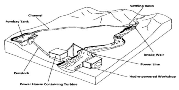
The diagram shows a typical micro-hydro scheme. Water from a stream or river is channelled into a tank and then released downhill through a pipe (or 'penstock'). When it reaches the bottom, the water drives a turbine that generates power. The amount of power produced depends on the distance the water falls before it hits the turbine and the number of litres per second flowing through the system. The turbine produces electricity or can be used to drive machinery directly.
