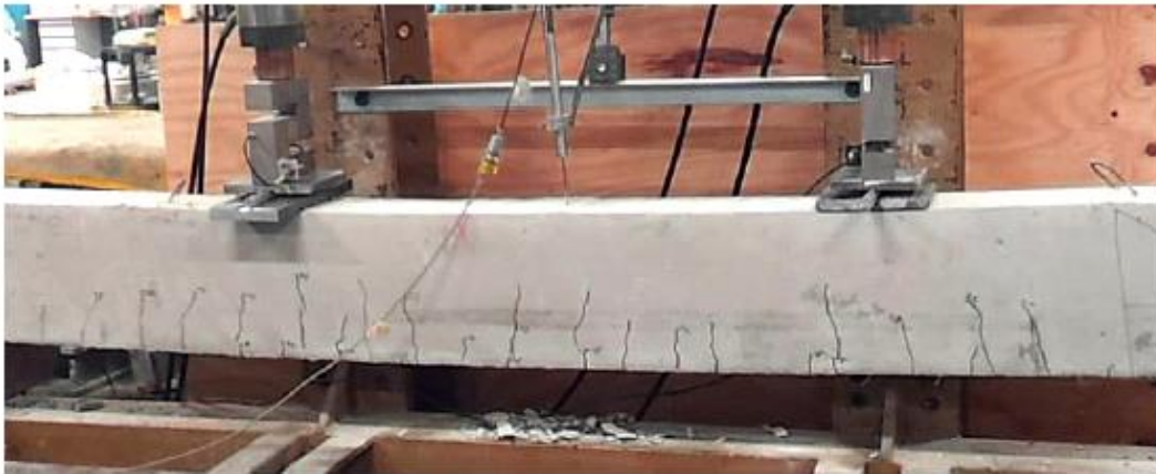
Vertical cracks are formed due to flexure, which are known as flexural crack
